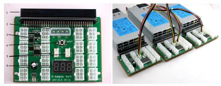
For every two X11 breakout boards, one 4-pin cable will be included to sync your power supplies together.
