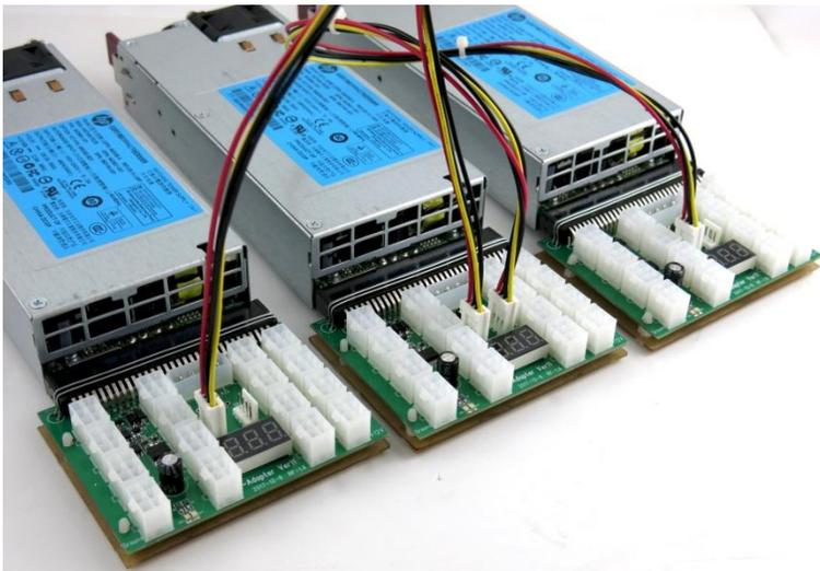
These breakout boards have two 4-pin input ports; you can sync any amount of power supplies together by connecting the 4-pin port to the next breakout board's 4-pin port and so on. We have tested up to 20 linked PSUs.
