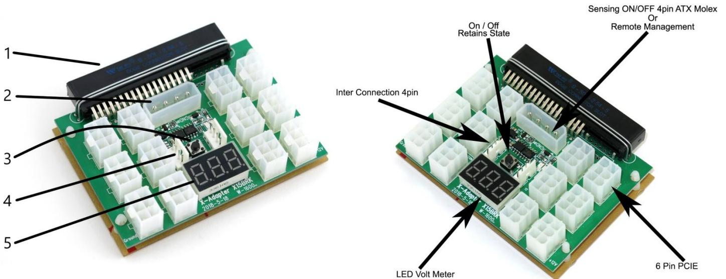
1: **Connector slot.** When connecting the breakout board to your PSU we recommend sliding in one corner of the slot from the PSU and then sliding the rest of the power bar into the connector slot. (Lubricant is not required, but recommended. Apply on the PSU power bar and wipe away any excess prior to connecting the adapter.)
